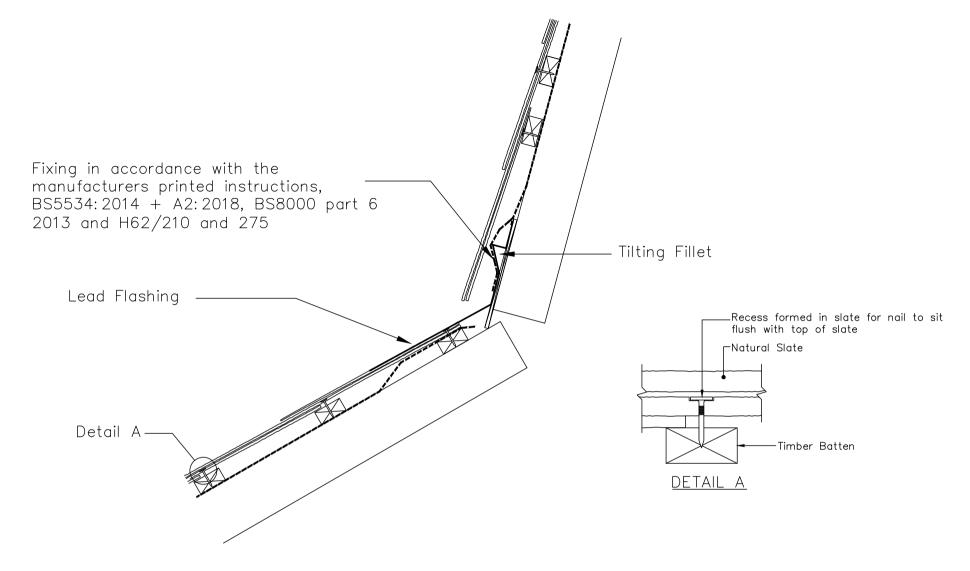
Grade slates into 3 or 4 groups of equal thickness. Sort slates in each group so that thin end of slates will be towards the ridge. Hole slates from the rear.
